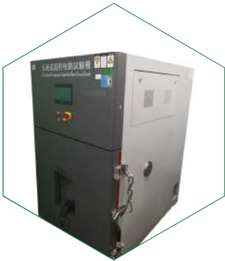
Short circuit Test
